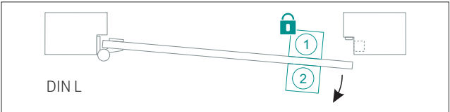
door DIN left handed, locking mechanism on the closing side
